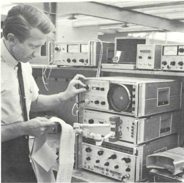
A complete s-parameter test setup good for frequencies up to 12 GHz includes an HP 8410A/ 8411A Network Analyzer ($4300) and an HP 8414A Polar Display ($1100), both housed in the top frame. In the center is an HP 8745A S-Parameter Test Set ($3000) and under it an HP 8690A Sweeper ($1600). If you are willing to sacrifice the con-
