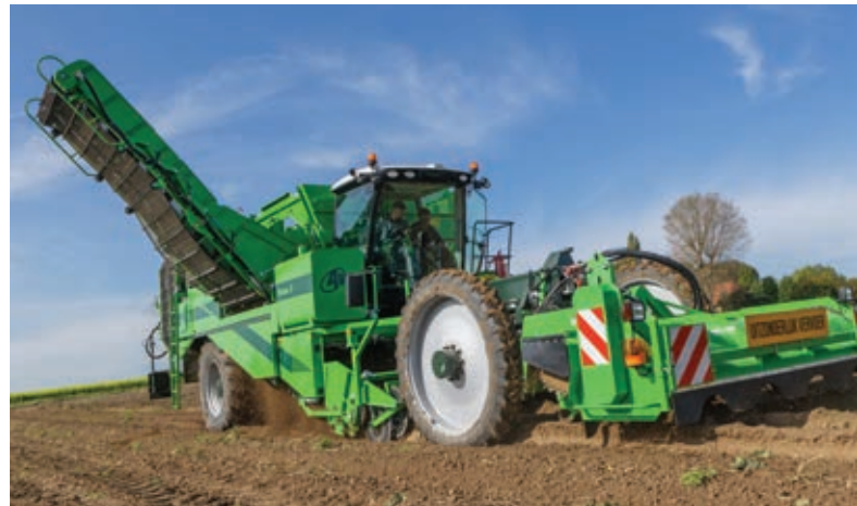
The Puma 3 from AVR can be equipped with attachments for harvesting potatoes, onions or carrots.
