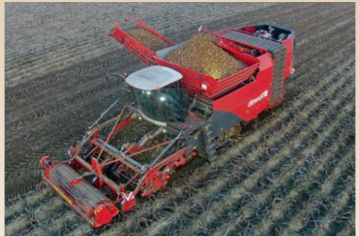
Dewulf's Kwatro Xtreme potato harvester lifts four rows at 90cm spacing.
