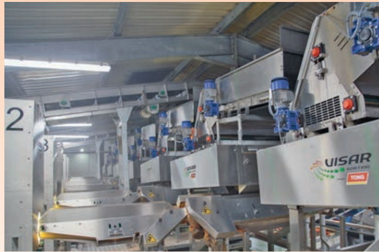
The new Tong grading system uses seven Visar optical graders which are capable of splitting the crop six-ways. They have increased crop utilisation while achieving a significant reduction in labour costs.
