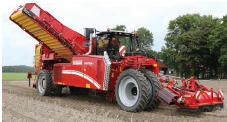
The Varitron Platinum two-row harvester features Grimme's recently introduced ErgoDrive control system.
