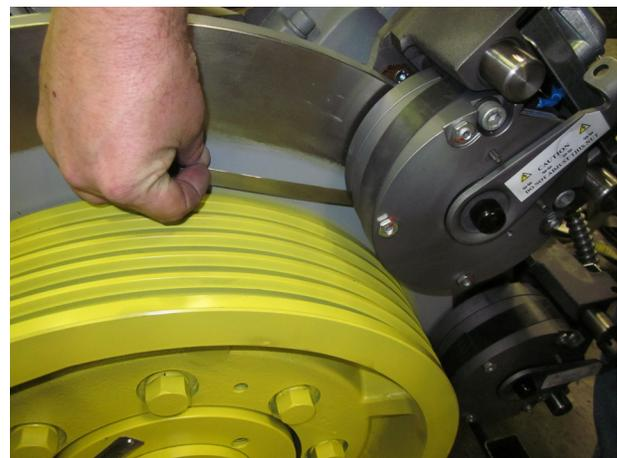
Figures 17: Check Brake Gap at 4 places around the brake to understand completely the brake position.
