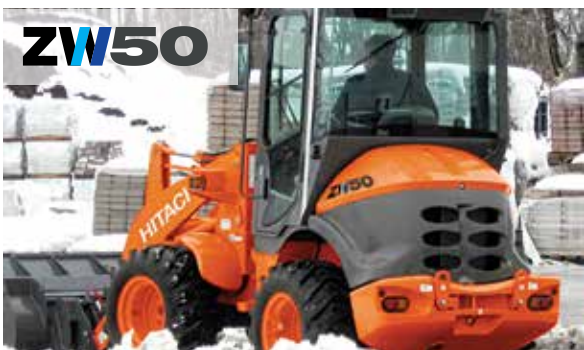
ZW50 Bucket Capacity . . . . . 0.8 yd 3 Operating Weight . . . . . 9,350 lbs Engine Output, Max, Gross . 44 HP Breakout Force . . . . . 5,530 lbs
