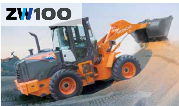
ZW100 Bucket Capacity . . . . . 1.7 yd 3 Operating Weight . . . . . 16,140 lbs Engine Output, Max, Gross . 101 HP Breakout Force . . . . . 13,730 lbs
