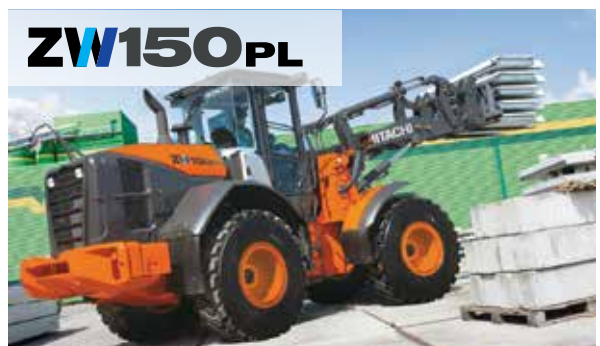
ZW150PL Bucket Capacity . . . . . 2.8 yd 3 Operating Weight . . . . . 27,010 lbs Engine Output, Max, Gross . 145 HP Breakout Force . . . . . 23,155 lbs
