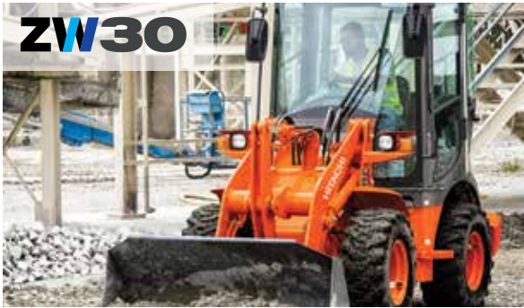
ZW30 Bucket Capacity . . . . . 0.52 yd 3 Operating Weight . . . . . 7,310 lbs Engine Output, Max, Gross . 25 HP Breakout Force . . . . . 4,630 lbs
