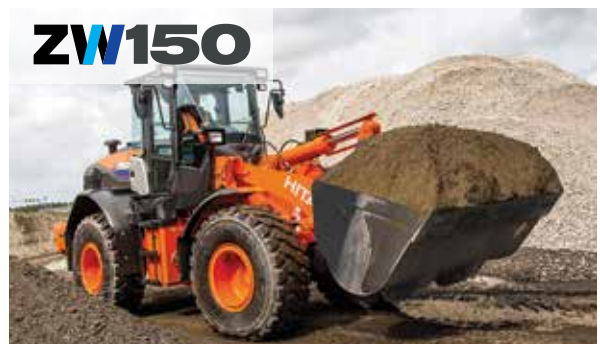
ZW150 Bucket Capacity . . . . . 3.1–3.5 yd 3 Operating Weight . . . . . 27,029 lbs Engine Output, Max, Gross . 145 HP Breakout Force . . . . . 22,481 lbs
