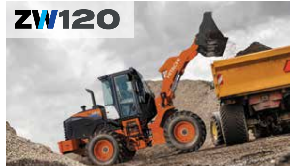
ZW120 Bucket Capacity . . . . . 2.0–2.4 yd 3 Operating Weight . . . . . 18,585 lbs Engine Output, Max, Gross . 99 HP Breakout Force . . . . . 16,840 lbs
