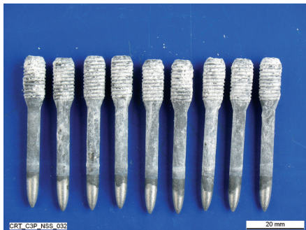
Zinc corrosion (white rust)
