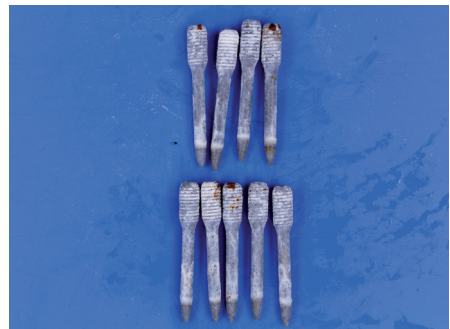
Start of carbon steel corrosion (red rust)
