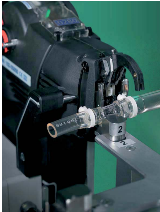
Exact positioning of cable ties.
