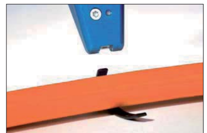
... release the push rod and remove the tool, the tie is cut.
