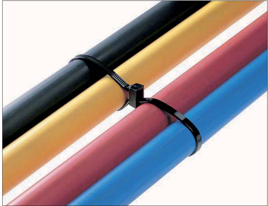
Parallel routing of two cable bundles using DH-Series. The double head creates an inside and an outside serrated loop.
