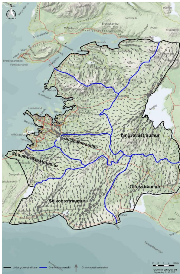
Figure 5.4.5 Calculated shallow groundwater flow in May 1980 when the groundwater divide reached furthest towards the north. The arrows show the direction of the groundwater flow (Vatnaskil, 2017).
