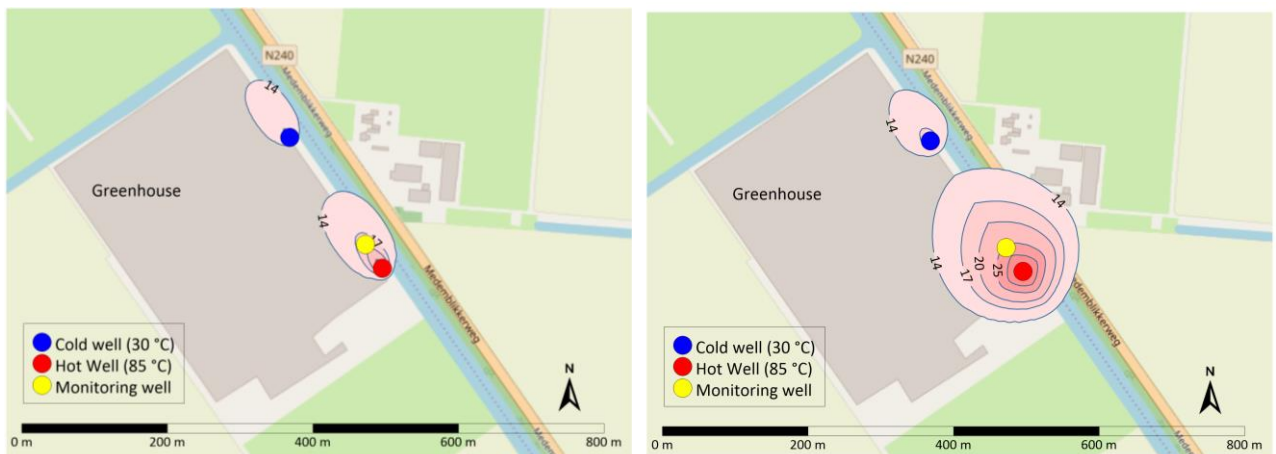
Figure 2.1.22 Top view of the temperature distribution at the middle (left hand side) and top (right hand side) of the 3 rd aquifer, after 20 years of heat storage with sand as backfilling material.
