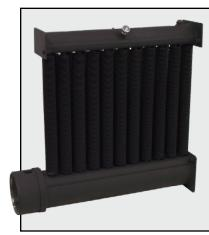
The *ExCaliber*<sup>™</sup> vacuum sealed liquid-to-air heat exchanger core is constructed using rugged, copper-free, roll-formed aluminum fins and protected by a pressure relief device, automatic reset high limit, and a back-up manual reset high limit.
