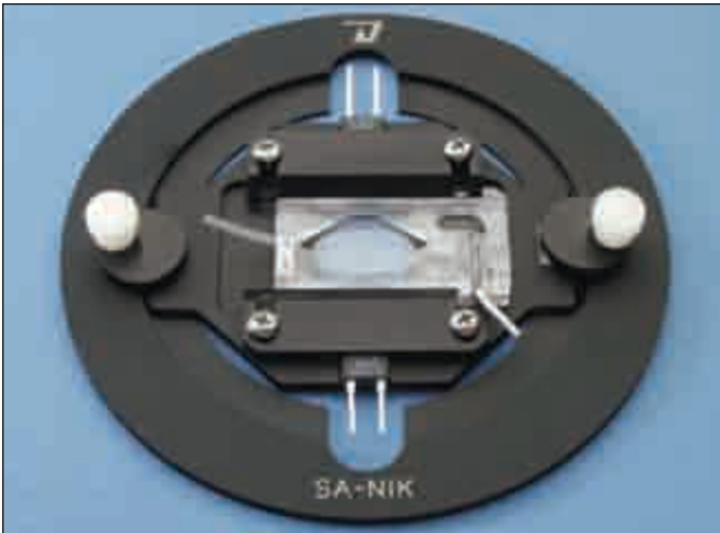
Model RC-26G chamber shown in a PH-1 heated platform on a stage adapter for a Nikon inverted microscope.
