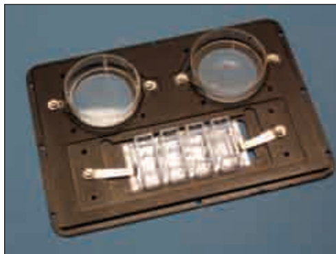
Plate adapter for Petri dishes and chamber slide
