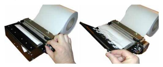
Figure 16 • Tear off the jamming paper against the fixed cutter blade.
