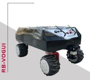
TUG CAPACITY: 680 KG AUTONOMOUS ALL TERRAIN ROBOT ROBOT AUTONOMY: UP TO 70 KM
