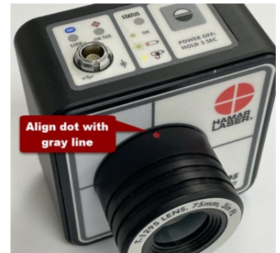
Figure 7 - T-1295/T-1296 Target with T-1295-AO-3 Lens installed correctly
