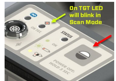
Figure 9 - T-1295/1296 Control Panel
