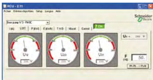
RCU: Remote Control Utility for communication tests.
