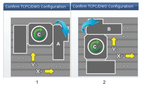
2. If your rotary configuration matches the diagram, press **[ENTER]** to confirm so. This activates TCPC/DWO.
