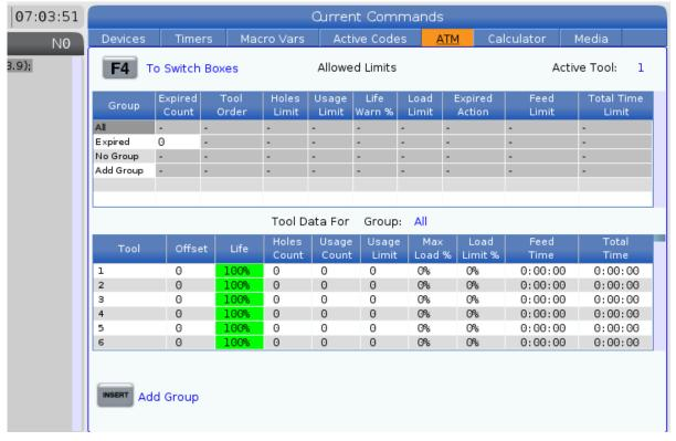
**Advanced Tool Management -**This page contains information the control uses to predict tool life. Here is where you create and manage tool groups, and where you enter the maximum tool load percentage expected for each tool.
