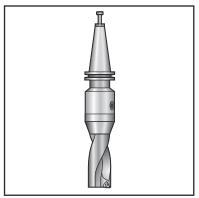
4. **Set pocket as Large [L]** - Use this flag when a large tool has a diameter of greater than 3" for 40-taper machines and greater than 4" for 50-taper machines. Scroll to the pocket of interest and press **[L]** to set the flag.
