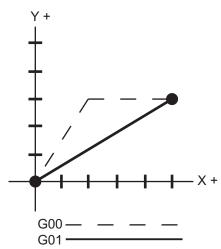
Setting 57 (Exact Stop Canned X-Y) can change how closely the machine waits for a precise stop before and after a rapid move.
