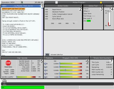
• Display boxes [1 - 7] are selectable. For example if you want to go to the Maintenance tab, press the coolant display box [4].
