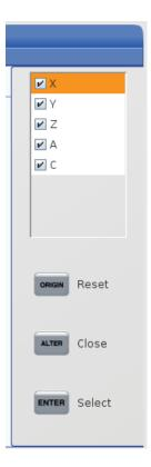
Use the cursor arrow keys to highlight an axis, and press **[ENTER]** to toggle it on and off for display. The positions display will show axes that have a check mark. Press **[ALTER]** to close the axis display selector.
