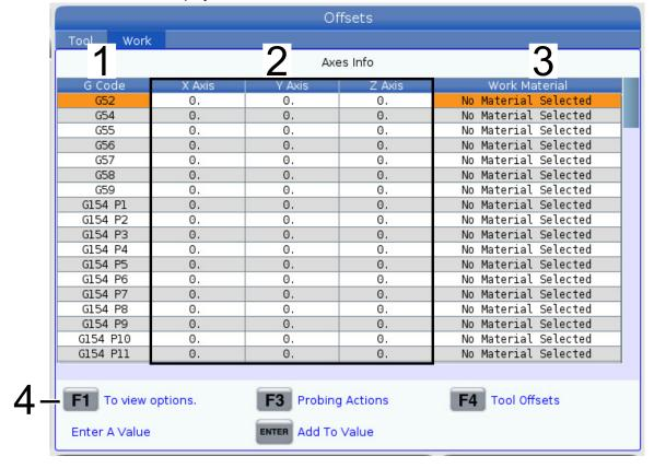
G Code - This column displays all the available work offset G-codes. For more information on these work offsets See "G52 Set Work Coordinate System (Group 00 or 12)" on page 344., See "G54-G59 Select Work Coordinate System #1 - #6 (Group
