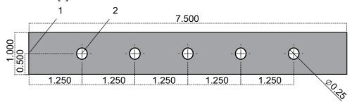
Below are two example programs that drill the holes as shown in the drawing, with a comparison between absolute and incremental positioning. We start the holes with a center drill, and finish drilling the holes with a 0.250" (6.35 mm) drill bit. We use a 0.200" (5.08 mm) depth of cut for the center drill and 1.00" (25.4 mm) depth of cut for the 0.250" drill. G81, Drill Canned Cycle, is used to drill the holes.
