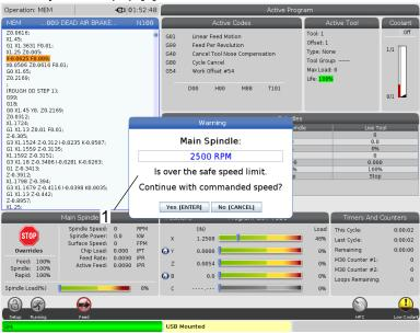
This feature will display a warning message when the **[FWD]** or **[REV]** button is pressed and the previous commanded spindle speed is above the Spindle Maximum Manual Speed parameter. Press **[ENTER]** to go to the previous commanded spindle speed or press **[CANCEL]** to cancel the action.
