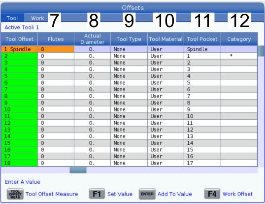
7. Flutes - When this column is set to the correct value, the control can calculate the correct Chip Load value displayed at the Main Spindle screen. The VPS feeds and speeds library will also use these values for calculations.
