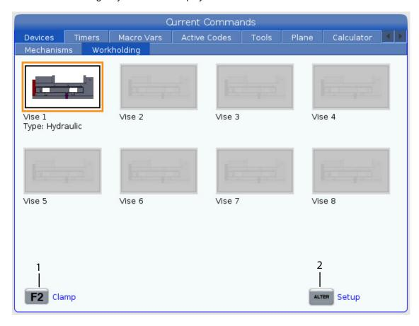
1. Clamp/Unclamp - Press **[F2]** to Clamp or Unclamp the Vise. In the program use M70 P1 to clamp and M71 P1 the vise. When commanding the M70 Pn / M71 Pn code the control will toggle an I/O output. Make sure the solenoid valve is connected to the correct output see the table below.
