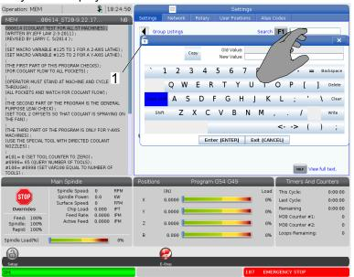
Press and hold any input line for the virtual keyboard to appear.
