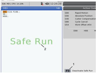
If your machine supports Safe Run, you will see a new icon in MDI with the text F3 Activate Safe Run [1]. Press [F3] to turn Safe Run on/off. Safe Run Active state is noted by a water mark [2] in the program panel.
