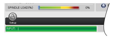
The input bar is the data entry section located in the bottom-left corner of the screen. This is where your input appears as you type it.
