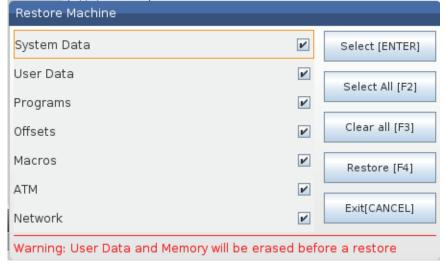
8. Highlight the data to restore and press **[ENTER]** to apply a check mark. Press **[F2]** to select all data. Press **[F3]** to clear all selectors.
