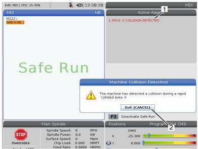
When a crash is detected, all motion is brought to a stop, an alarm [1] is thrown, and a popup [2] is generated letting the operator know that a crash was detected, and which axis it was detected on. This alarm can be cleared by **[RESET]**.
