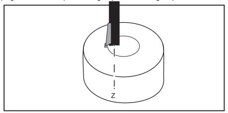
Spindle orient command M19 P/R code which used to position the spindle before broaching must be used first before executing G156 broaching canned cycle.
