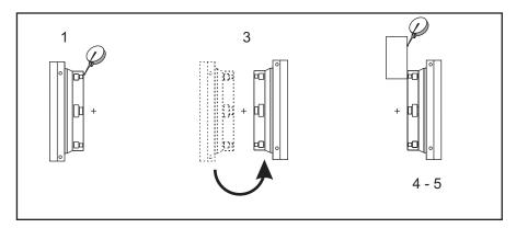
1. Jog the tilt axis until the rotary platter is vertical. Attach a dial indicator to the machine spindle (or other surface independent of table motion) and indicate the platter face. Set the dial indicator to zero.
