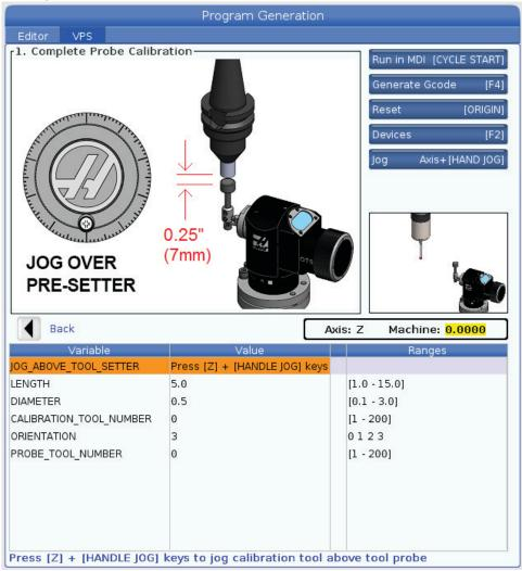
To calibrate the tool probe:
