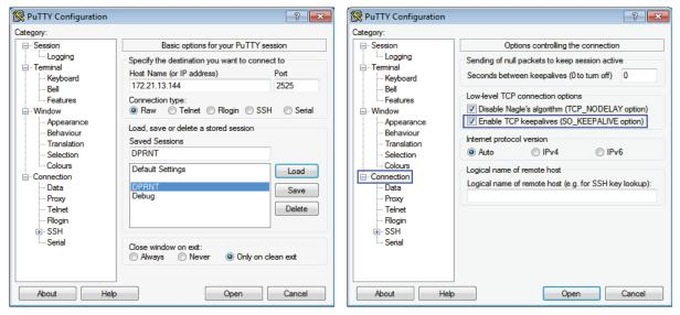
To check the connection, type <code>?Q100</code> in the PuTTY terminal window. If the connection is active, the machine control responds with <code>SERIAL NUMBER</code>, <code>XXXXXXX</code>, where <code>XXXXXXX</code> is the machine's actual serial number.
