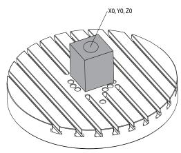
In the figure below, the actual workpiece is not located in this programmed position. The center of the workpiece is actually located at X3, Y-2, Z0, and is defined as G54.
