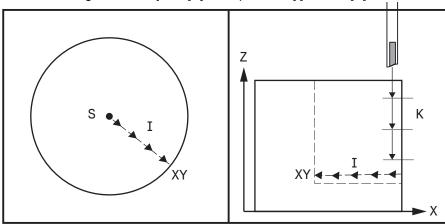
Broaching operations canned cycle can be done on Inner and outer grooves in different position using the G156 code with an optional address codes which define the tool Pecks and the cut paths.
