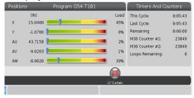
When the light curtain beam is obstructed the machine will go into a Light Curtain Hold condition and the Light Curtain icon will appear on the screen. The icon will disappear when the beam is no longer obstructed.
