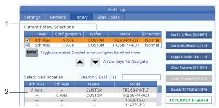
The custom rotary configurations appear as options in the Select New Rotaries table. You can select them in the same way you would select a base rotary configuration. You can also save more than one custom configuration for the same rotary unit:
