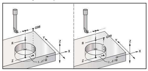
In addition to boring the hole, this cycle will shift the X and/or Y Axis prior to retracting in order to clear the tool while exiting the part. If  $\mathbb Q$  is used Setting 27 determines the shift direction. If  $\mathbb Q$  is not specified, the optional  $\mathbb I$  and  $\mathbb J$  values are used to determine the shift direction and distance.
