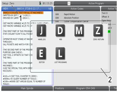
• Press the upper left corner [1] of the screen to have the operation mode panel popup box [2] to appear. Press the mode icon to put the machine in that mode.
