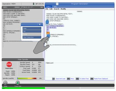
• In edit mode you can drag your fingers across the code to use the handle bars to copy, cut and paste a section of the program.
