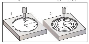
These G codes assume cutter compensation, so you do not need to program G41 or G42 in the program block. However, you must include a D offset number, for cutter radius or diameter, to adjust the circle diameter.
