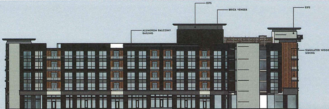
REAR ELEVATION- APARTMENT BUILDING
