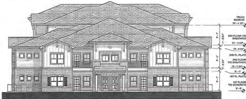
4 BUILDING TYPE III LEFT ELEVATION 1/8" = 1'-0"
