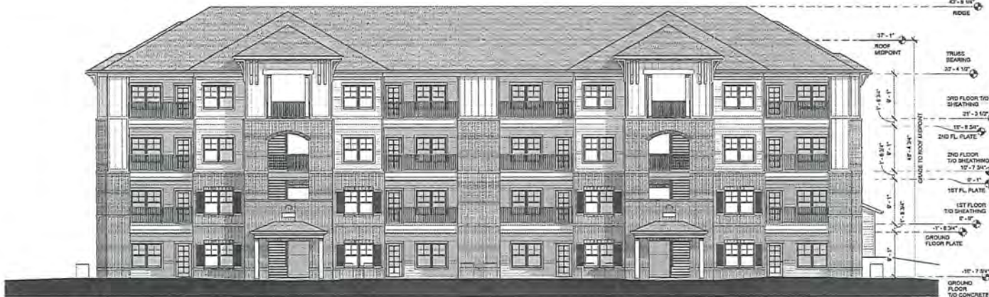
2 BUILDING TYPE I FRONT ELEVATION 1/8" = 1'-0"
