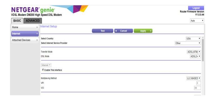
DSL Mode - ADSL2+ Transfer Mode - ADSL(ATM) Multiplexing Method - Leave Default - LCC-BASED VPI - 0 VCI - 35
