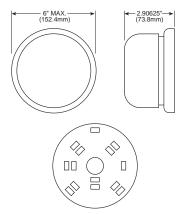
Universal adaptaplate mounts directly on surface of any single gang opening: 3 1/4," 3 1/2", 4" octagon; 4" SQ. box or equivalent surface fitting. Sound level: 92 dB at 10'. Weight: 2 lbs. 11 oz. (1.2 kg)
