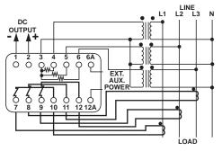
E Models: Shown S Models: External auxiliary power not required. Bottom terminal strip (7-12) omitted on S-model 1-element units
