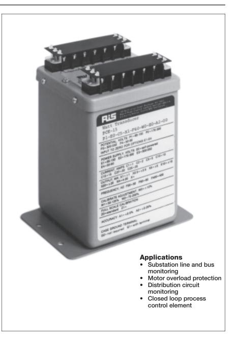
The Ametek Power Instruments Watt and VAR transducers provide a Direct Current (DC) output proportional to the real or reactive power input. The output accuracy is 0.25% including the effects of current, voltage, power factor, frequency, and output load.
