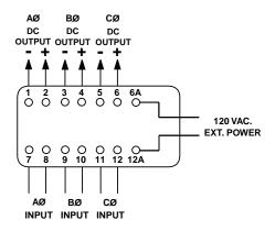
E Models: Shown S Models: External auxiliary power not required. Bottom terminal strip (7-12) omitted on S-model 1-element units
