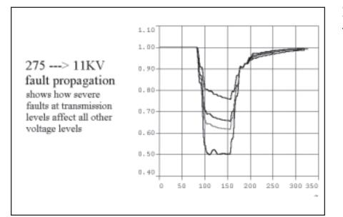
Voltage Fault Propagation Comparing Voltage Dip Severity at Different Power System Voltage Levels
