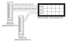
Multiple Remotes With Outputs To One Common Annunciator Window
