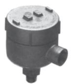
The Ametek Model VT-3360 Vibration Transmitter is a totally solid-state device providing vibration monitoring for non-critical rotating machinery. It combines a vibration sensor and electronics that provide for input power, 4-20 mA analog vibration output signal, and 0-1.0 mA vibration wave form output signal-all on just two wires. Various adjustments, sensing ranges and other features make the VT-3360 suitable for many vibration monitoring applications.
