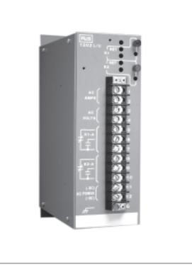
These single and dual trip alarms accept AC current or voltage inputs (field alterable) and provide one DPDT 5 amp (ET-1200L/U or two SPDT 5 amp (ET-1202L/U) universal relay contact outputs. Basic input spans are 16 to 200 VAC or 0-1 to 0-7.5 amps.
