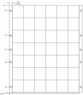
Panel Mounting All mounting dimensions are based on the number of cells, not windows. Each cell can be divided into up to 4 windows.
