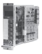
VT-2466-TK tachometer modules provide continuous monitoring of shaft speed (RPM) when used in Ametek Series VT-2490 machine monitoring systems. Each features its own independent, continuous digital display of shaft speed from 0.1 to 19,999 RPM in large easy-to-read digits. A Ametek tachometer module accepts an input from a proximity probe, magnetic pick-up or a fiber optic light source and provides power to the sensor as needed.
