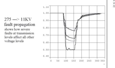
Voltage Fault Propagation Comparing Voltage Dip Severity at Different Power System Voltage Levels
