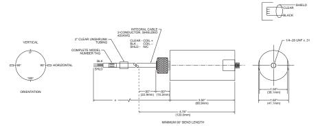
Velocity Pickup Model 1722V
