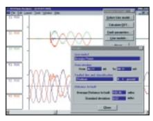
Event Waveform Display Window, with fault location results identified.
