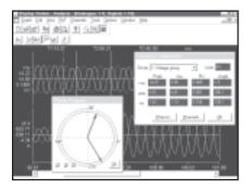
Event Waveform Display Window, with the Power Analysis Toolkit active. Sequence Components calculated on a Phase Group basis. A Phasor Diagram is also displayed with the angle based on the start of the selected region.
