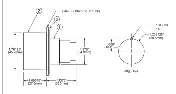
NOTE: Contact Rating: Continuous, 10 A Normal Load Break: 120 VAC, 6 A or 125 VDC 2.2 A. Weight: 6 oz. (.2 kg)
