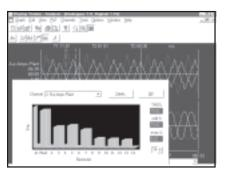
Event Waveform Display Window, with the Power Analysis Toolkit active. Harmonic Analysis on any channel over a selected time frame.
