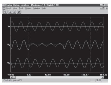
Waveform Capture (simultaneous on up to 16 analog and 32 digital inputs)
