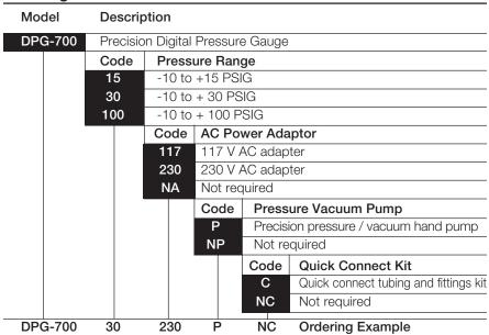
DPG-700 precision digital pressure gauge, measuring pressures in the range -10 to +30 PSIG, with 230 VAC power adapter and precision hand pump.
