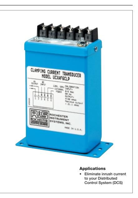
Ametek introduces a new current limiting 4-20 mAdc Current Transducer that clamps the output to 21.1 mAdc with current overload. This current limiting feature is ideal for all Distributed Control System (DCS) applications where inrush current can cause the DCS to misinterpret the signal resulting in equipment failure or erroneous system operation.
