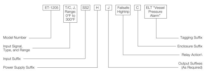
This order is for a Model ET-1205 thermocouple alarm which accepts a Type IJ thermocouple with a range of 0°F to 300°F. The input span is between 5 and 9.99 mV (SS2). The alarm features 24Vdc prime power (H), two SPDT hermetically
