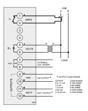
11/2-Element Watt, Var, Watt/Var with External Aux. Power
