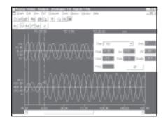
Event Waveform Display Window, with the Power Analysis Toolkit active. Single Channel Calculations made on any channel over a selected time frame.
