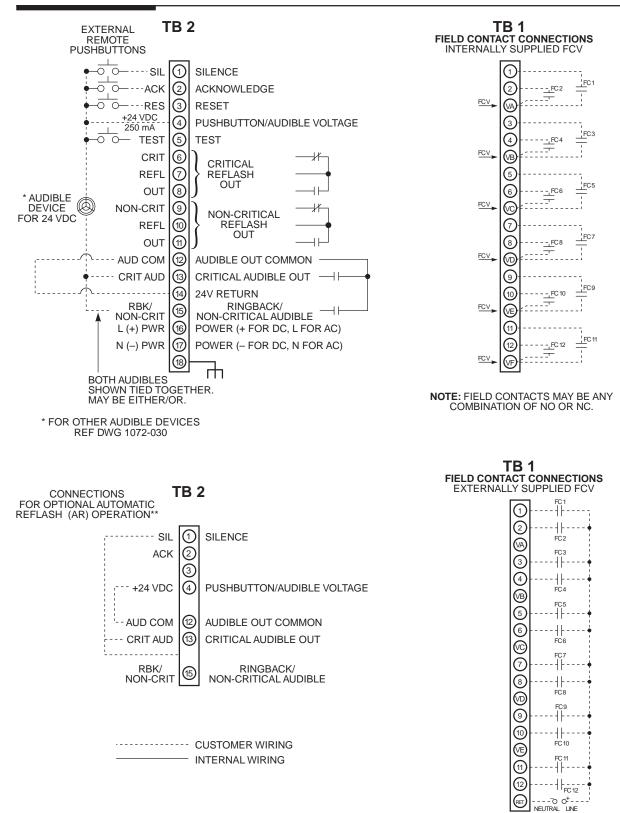
\*\* Recommended configuration for remote AN-3196B reflash output to main annunciator, where audible function in remote location is not required. This hook-up is not compatible with audible device hook-up shown in above diagram.
