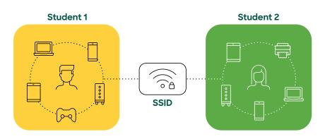
WPN allows all user devices to authenticate to the SSID and communicate, creating a personal network
