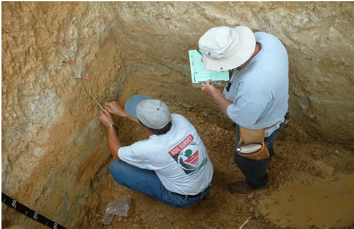
Fig. 2. Soil horizons or zones of uniform morphological characteristics are identified for sampling.
