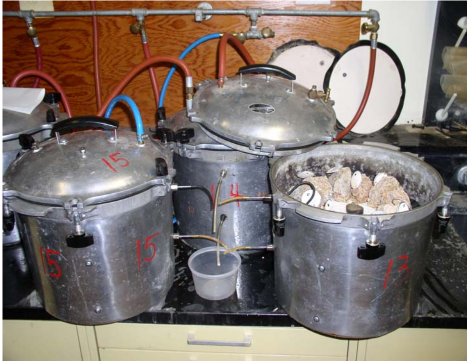
Fig 1. Clods placed in pressure-plate extractor following saturation.
