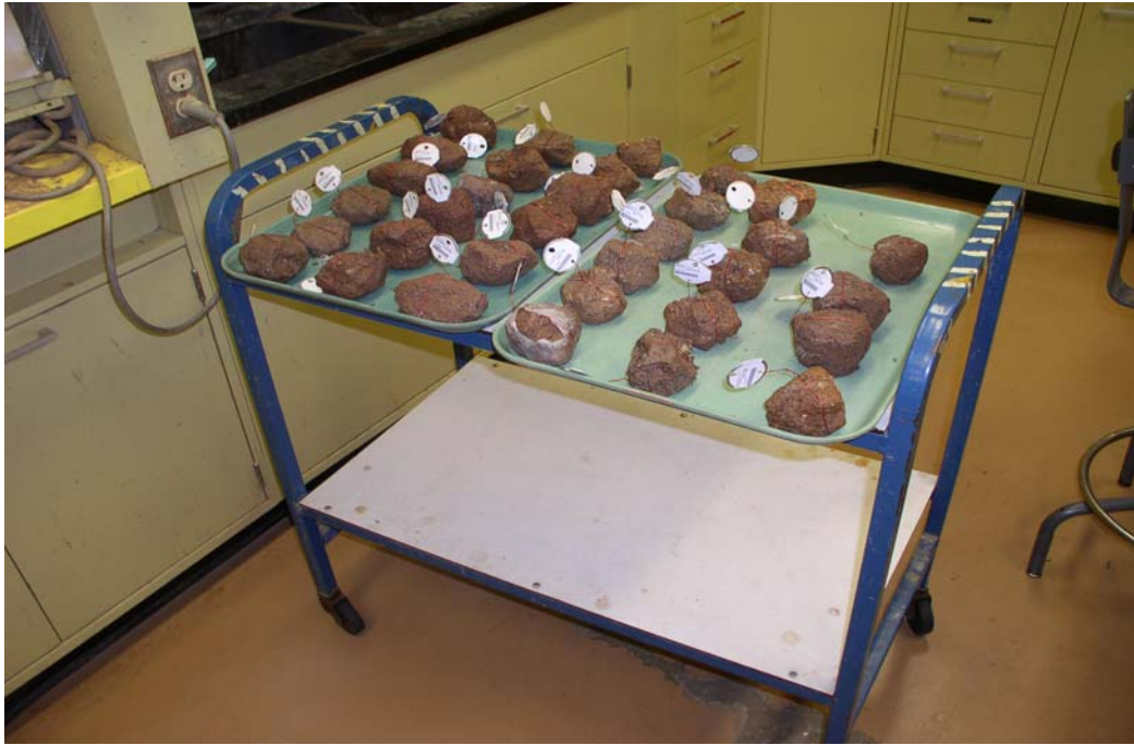
Fig. 1. A round stock tag with sample identification number is prepared. The cut copper wire is looped around the clod.
