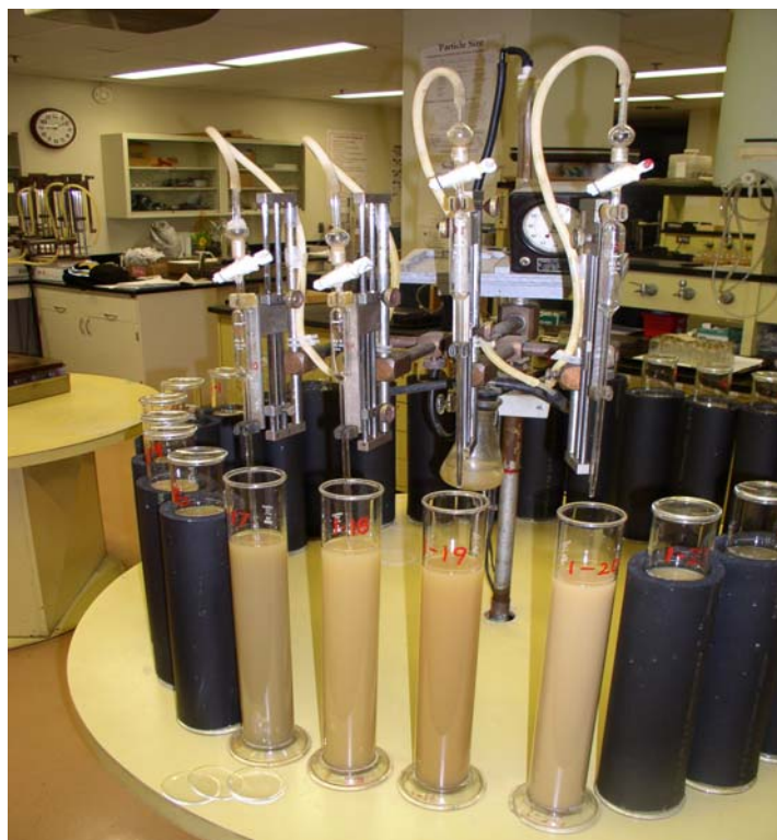
Fig. 3. Shaw Pipet used for particle-size analysis of the <2-mm fraction at the USDA-NRCS Soil Survey Laboratory.
