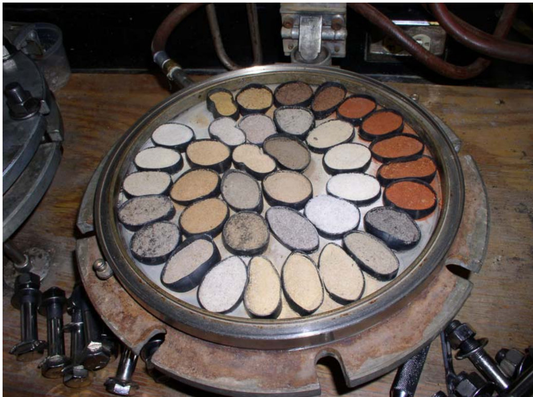
Figure 2. Pressure-membrane extraction at 1500-kPa for <2-mm samples.
