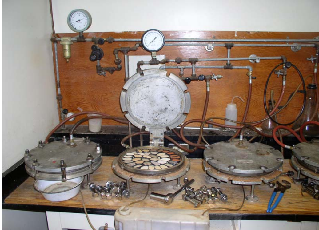
Figure 1. Sieved (<2-mm) soil placed in pressure-membrane extractor.
