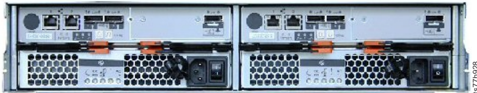
Figure 24. TS7740 Cache Controller 3956-CC9 (rear view)
