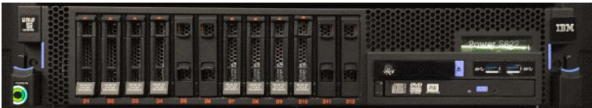
Figure 7. TS7700 Server (3957-VEC) System Unit (front view)
