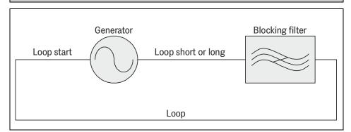
If an energy track (20 kHz, 25 kHz or 141 kHz) is used in combination with a normal inductive loop (guide wire, frequency in the range of 5 .. 10 kHz) it can happen that the energy track induces a voltage into the guide wire loop. This voltage results in a current in the loop that can influence the generator's current regulation or - in extreme cases – destroy the generator.
