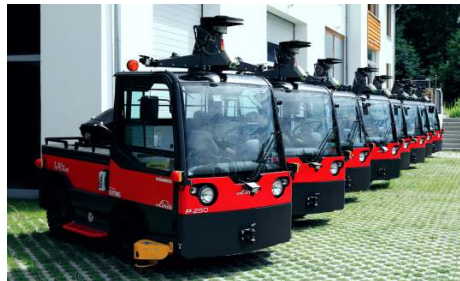
Automated electric tow tractors with automatic coupling and uncoupling of trailers
