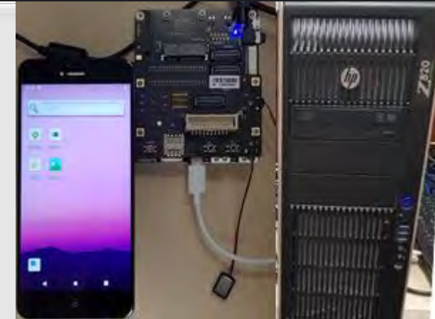
Qualcomm Development Board connected to (mcmurdo) HPZ820
