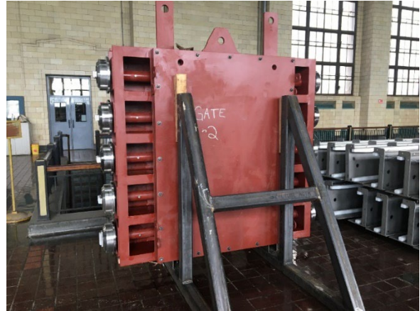
New Low Lift suction isolation gate
