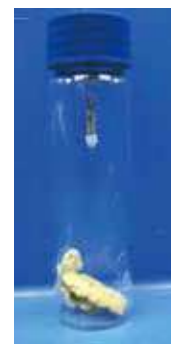
Sampling blue cheese with MonoTrap RGPS TD
