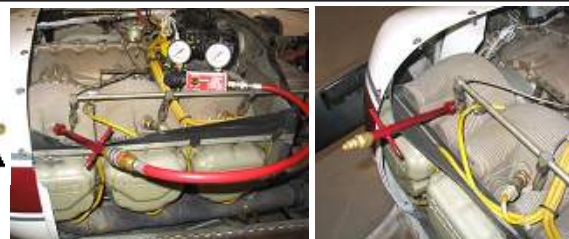
Compression Tester Extension is not FAA-PMA approved.
