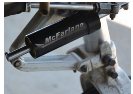
P/N MC0442512-1 installed on a 152
