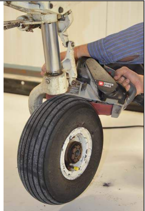
Use a belt sander to remove the shimmy wear pattern in the tread.
