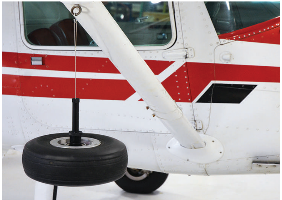
Use wheel balancer P/N TOOL128 for 3/4" diameter axles or P/N TOOL129 for 1", 1 1/4", and 1 1/2" axles to check tire for proper balance (additional sizes available). See page 263 for additional information.
