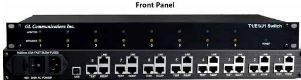
Back Panel T1/E1/J1 Monitor /Intrusive Switch
