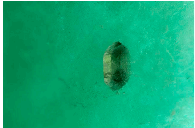
Figure 13. This doubly terminated tetragonal crystal in jadeite jade was identified as “high” zircon using Raman spectroscopy. Photomicrograph by Tyler Smith; field of view 2.90 mm.
