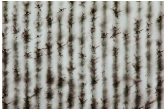
Figure 13. The internal growth zonation was composed of a regular network of small crack clusters around a central black point, presumably due to laser impact. Photomicrograph by Yu-Ho Li; field of view 2.14 mm.
