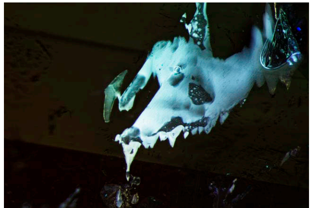
Figure 6. When the same inclusion scene is lit with a long-wave ultraviolet flashlight, it becomes evident that the cavity contains a filler that fluoresces a chalky blue color in long-wave illumination. The irregular shapes can also be seen to contain rounded gas bubbles. Photomicrograph by E. Billie Hughes; field of view 4 mm.
