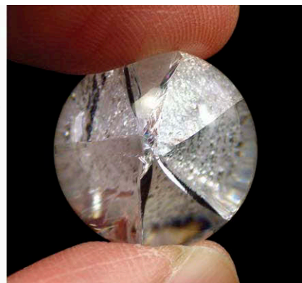
Figure 14. Left to right: A schematic diagram, a bottom view, and a top view of an imitation phantom crystal. The six fractures (red dashed lines) along the ridgeline of the pseudo-hexagonal pyramid in this imitation phantom quartz sphere were reportedly formed without any external force or heat treatment. The diameter of this sphere is 17.68 mm. Photos by Shu-Hong Lin.
