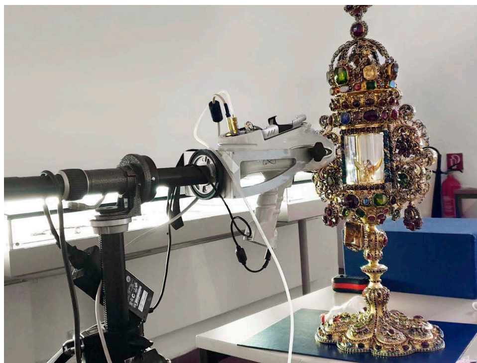
Figure 12. Gemstones decorating the Limburg pieces, such as the monstrance shown here, were identified using energy-dispersive X-ray fluorescence (EDXRF) spectroscopy. Photo by H.A. Gilg.
