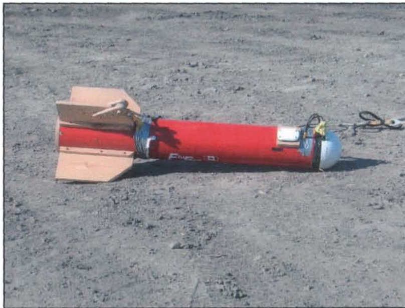
Figure 5: Geometrics cesium magnetometer mounted in the towed-bird airfoil.
