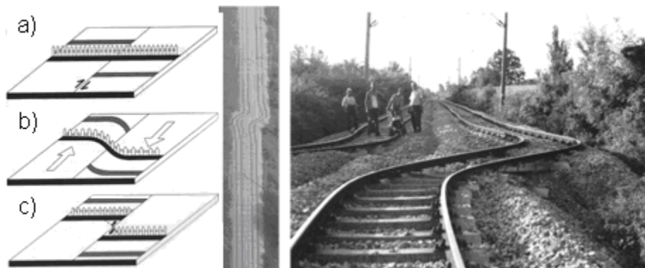
Figure 1.2 Illustration of the elastic rebound model. Left: The arrows show the relative motion across the fault. (b) When the two sides move and the fault is locked, the material on the two sides of the fault undergoes complete elastic deformation and linear features in (a) become deformed. (c) finally the strain becomes so large that the fault slips and we have an earthquake. The deformed material rebounds to its original position and features across the fault are offset. Figure from Stein and Wysession (2003) and copied from http://epscx.wustl.edu/seismology/book/book_no_captions/figures/ . Right: Displaced railroad tracks due to an earthquake. The earthquake causing this displacement was the 1999 Izmit earthquake of magnitude 7.4 (pictures from Aykut Barka).
