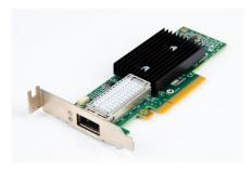
Mellanox MCX353A-FCCT ConnectX-3 Pro VPI adapter card, single-port QSFP, FDR IB (56Gb/s) and 40/56GbE, PCIe3.0 x8 8GT/s, tall bracket, RoHS R6
