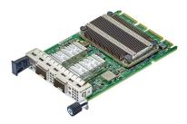
Broadcom BCM957414N4140C N225P Dual-Port 25/10 Gb/s Ethernet PCIe 3.0 x8 OCP 3.0 SFP Network Adapter BCM957414N4140C
