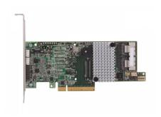
Broadcom LSI 9266-8i LSI00295 PCIe 2.0 x8 LSISAS2208 8 Internal Ports 6Gb/s SATA SAS RAID Controller 9266-8i
