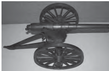
Unique Arsenal Model of Armstrong Breech Loader with Gravity Return Carriage
