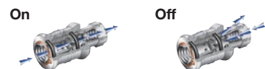
ON: In the "on" or open position, pressure flows from the inlet through a series of radial holes in the body to the air circuit
