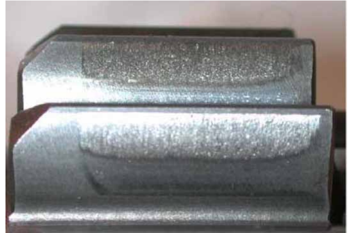
Figure 6 Scuffed gear set from dynamometer test.
