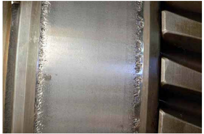
Figure 16 Micropitting on CRB IR of wind turbine HS pinion.
