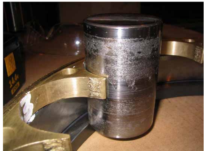
Figure 18 Scuffing on CRB roller from wind turbine INT pinion bearing.
