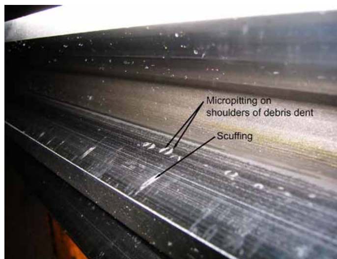
Figure 11 Wind turbine sun pinion with micropitting on shoulders of debris dents.
