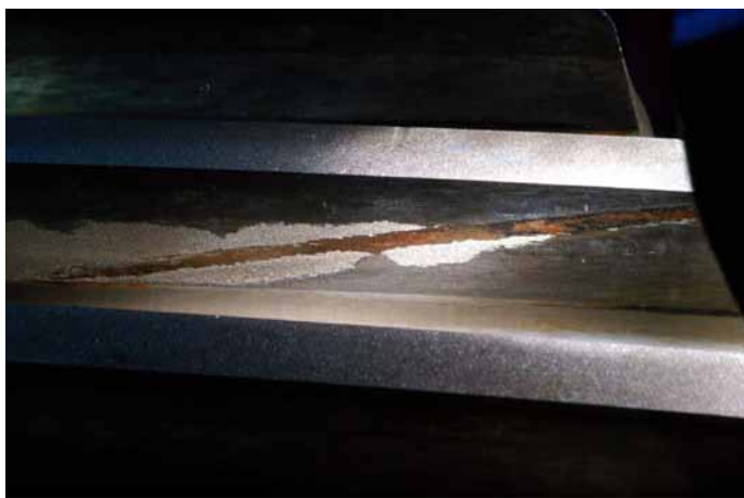
Figure 15 Wind turbine INT wheel with micropitting at edges of fretting line.
