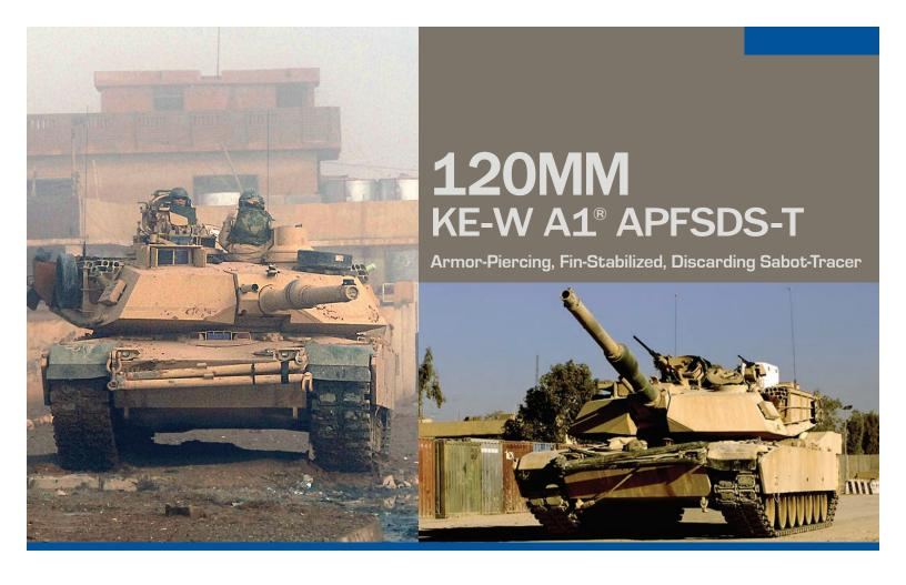
The 120mm KE-W A1® cartridge has been developed to provide state-of-the-art tungsten Armor-Piercing, Fin-Stabilized, Discarding Sabot-Tracer (APFSDS-T) cartridges for 120mm smoothbore cannons.
