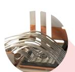
**Long lifetime** Wire bonding technology for lower thermal and mechanical stresses on power chips
