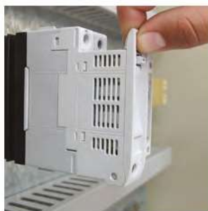
1. Preparation for opening fuse holder
