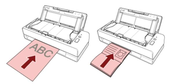
The document is pulled in and set inside the scanner when inserting the document into the return path opening.
