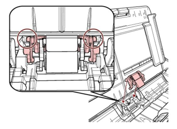
Attach the pad unit so that the protrusions are placed as shown below.
