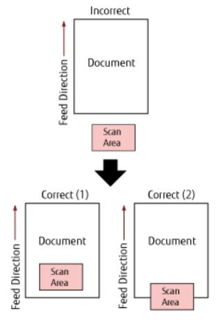
Outside of the document may have been scanned because the scanned document is shorter than the specified paper size. Take one of the following measures, and then scan again.
