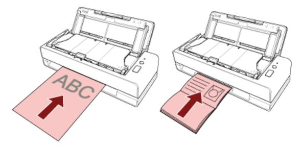
• For the ADF paper chute (feeder) Face the front side (scanning side) of a document upwards and load the top end of the document headfirst.
