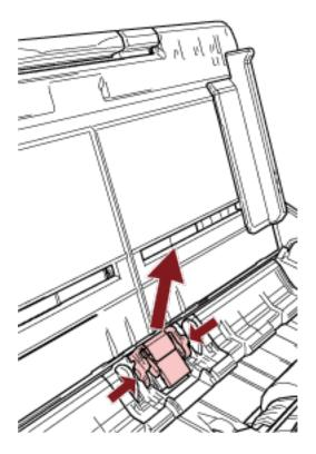
Squeeze both ends of the pad unit (gray parts) and pull it out in the direction of the arrow.
