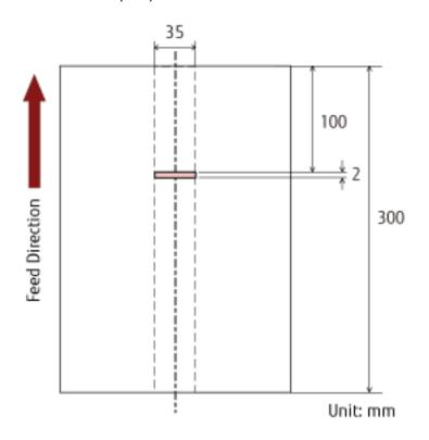
Since the detection area (length) is less than 5 mm, overlapped documents cannot be detected accurately.
