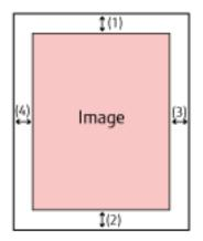
(1): Top = 0 to 15 mm (2): Bottom = -7 to 7 mm (3): Right = 0 to 15 mm (4): Left = 0 to 15 mm
