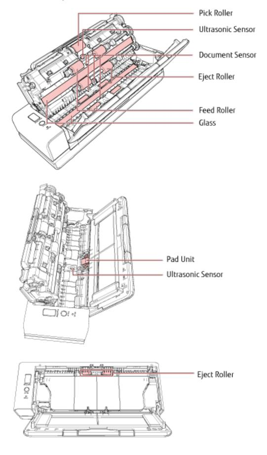
4 Clean the following locations with a cloth moistened with Cleaner F1, or a sheet of Cleaning Wipe.
