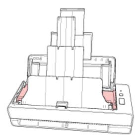
When a paper jam does not occur, completely push in the extended stacker by hand and close the stacker manually.
