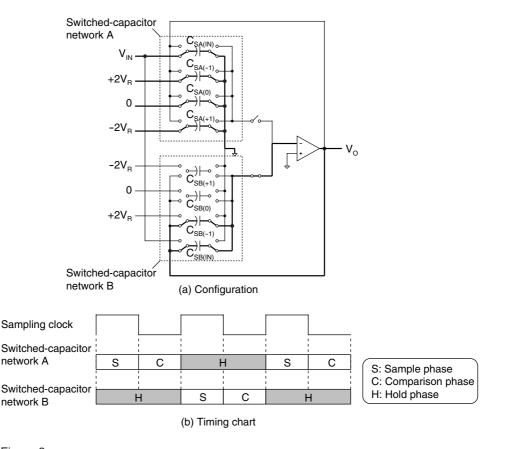
Figure 8 Configuration and timing chart of double-sampling FADAC.
