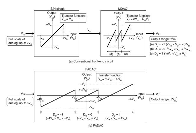
Figure 6 Comparison of transfer functions.
