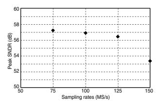
Figure 14 Measured Peak SNDR versus sampling rates at 2 MHz sinusoidal input.
