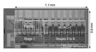
Figure 10 ADC chip photomicrograph.
