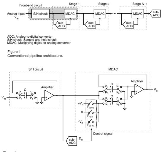
Figure 2 Conventional front-end circuit.
