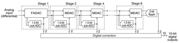
Figure 7 Block diagram of prototype ADC.
