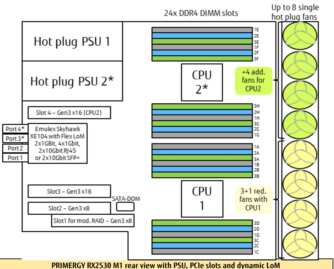
PRIMERGY RX2530 M1 rear view with PSU, PCIe slots and dynamic LoM
