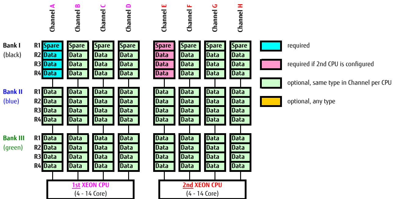
Rank Sparing Mode requires identical modules (same capacity and technology) within the same channel. The available memory for applications will vary depending on configuration. Please refer to the spreadsheet above "Effective Memory capacity with active Rank Spared Mode". Population rule for Rank sparing mode is to achieve max. available memory, e.g. 6 DIMMs will be spread across two channels, each with 3DPC
