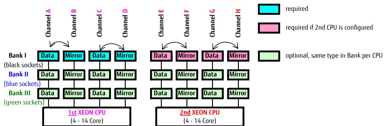
Mirrored Channel Mode requires identical modules on channel A,B, C, D (1st CPU) or channel E, F, G and H (2nd CPU) 50% of the capacity is used for the mirror => the available memory for applications is only half of the installed memory. If this mode is used, a multiple of 4 identical modules has to be ordered.
