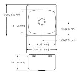
Single compartment self rimming topmount sink with faucet ledge. 18 gauge (1.2 mm), type 316 (EN 1.4401 17/12/2) stainless steel. Exposed surfaces are #4 satin finished. Undercoated to reduce condensation and resonance. Includes waste fitting, factory applied rim seal, cutout template, and factory installed EZ TORQUE™ fasteners. Certified to ASME A112.19.3-2008 / CSA B45.4-08.
