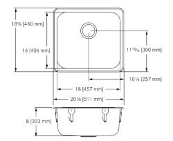
Single compartment self rimming topmount sink less faucet ledge. 18 gauge (1.2 mm), type 316 (EN1.4401 17/12/2) stainless steel. Exposed surfaces are #4 satin finished. Undercoated to reduce condensation and resonance. Includes waste fitting, factory applied rim seal, cutout template, and factory installed EZ TORQUE™ fasteners. Certified to ASME A112.19.3-2008 / CSA B45.4-08.
