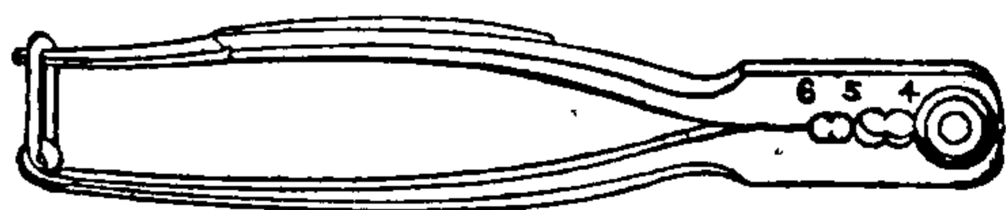
Fig. 321. Twisting Clamp for McIntire's Parallel Joint.
