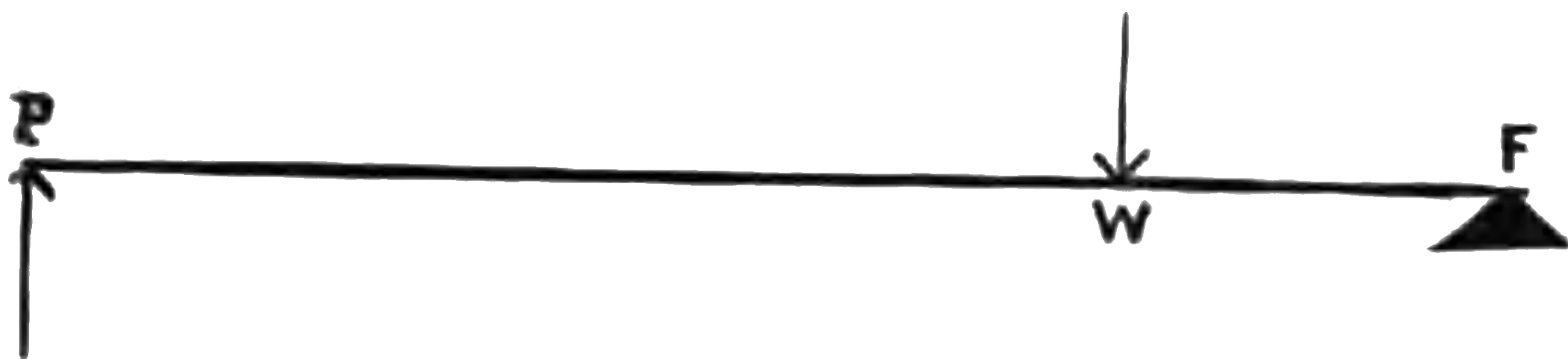
FIG. 57.—A lever of the second order. F , fulcrum; P , power; W , weight. The arrows indicate the direction in which the forces act.
