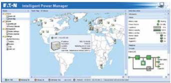
IPM scales easily from a local area network to a global view, keeping an eye on power conditions and equipment status. In addition to the default maps, it's possible to upload more maps, floor plans and other images. There can be separate views for multiple geographical areas and buildings.
