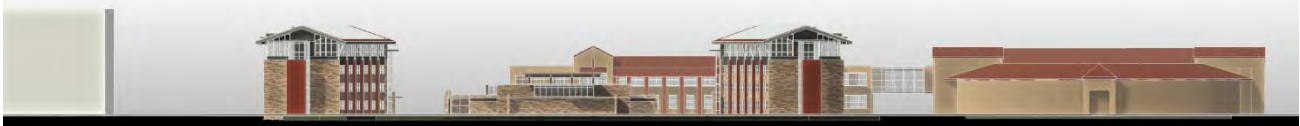
Concept sketch indicating a four-story massing, proportional and material studies with existing arcades removed and in context with surrounding buildings.
