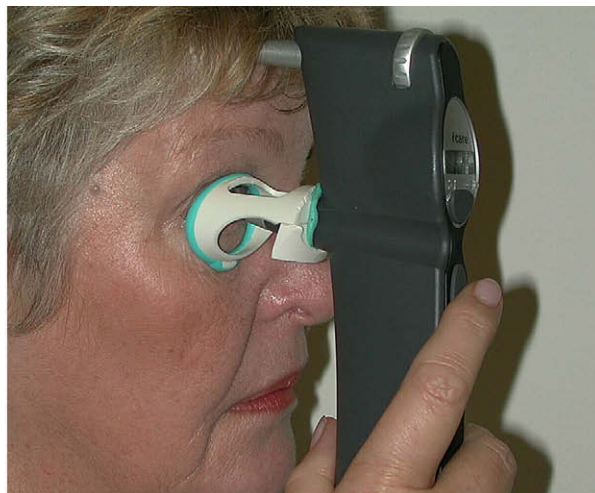
Fig. 7. (Left and Right): The ICare rebound tonometer (Tiolat, Finland) and technique of self-measurement using a lid-holder and positioning device.
