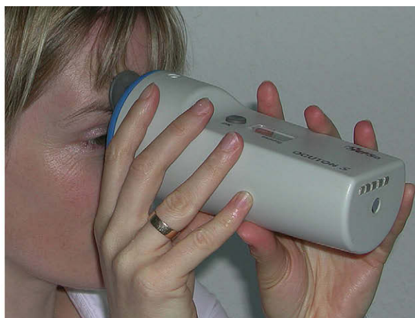
Fig. 2. (Left and Right): The Ocuton S tonometer (EPSa Elektronik & Präzisionsbau, Saalfeld, Germany). Reprinted with permission from EPSa Elektronik.
